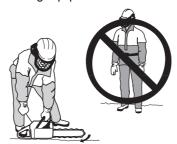
Place the chain saw on the ground and hold the rear handle down with your right foot. Grasp the front handle firmly using your left hand. Make sure the chain saw is steady and the chain is not touching the ground or other
